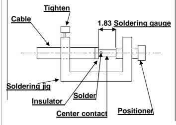
After cooling remove cable assembly from the jig. Insert cable+centre contact in the connector.
