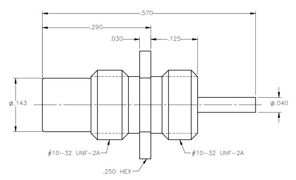
NOTES: LEAK RATE LESS THAN 1x10^-8 cc/sec AT A DIFFERENTIAL PRESSURE OF 15 PSI. MATERIALS:
