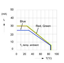
Ambient Temperature vs. Allowable Forward Current
