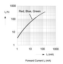
Fig.2 Relative Luminous Intensity vs. Forward Current
