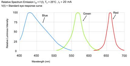
Fig.1 Relative Luminous Intensity vs. Wavelength
