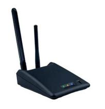
Bivar's Wireless Gateway Communication Center (BWGCC) is configured to receive and aggregate peripheral sensor information and manage corresponding sensors. The main function of the BWGCC is to forward the data from each Bivar Smart Device to the Bivar Cloud Server.
