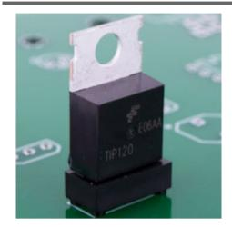
PERM-O-PADS, Square, TO-5 to TO-18, T-1 3/4 LED, Universal, 4 Lead, W/Open Center, 0.24 Length, 0.24 Width, 0.10 Thick, Nylon, White
