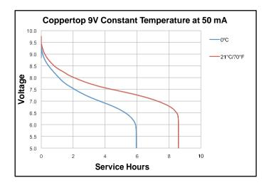
Delivered capacity is dependent on the applied load, operating temperature and cut-off voltage. Please refer to the charts and discharge data shown for examples of the energy/service life that the battery will provide for various load conditions.
