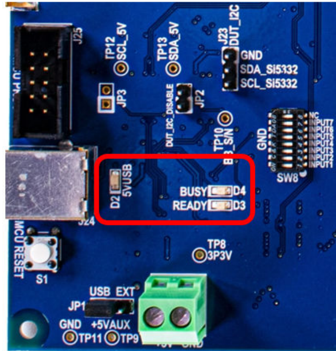
Figure 3.2. Si5332-8A-EVB LED Locations
