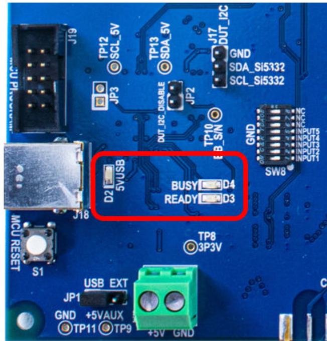
Figure 3.2. Si5332-6A-EVB LED Locations
