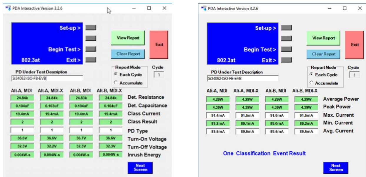
Figure 4.1. Si34062-ISO-FB-EVB PD SIFOS PoE Compatibility Test Results
