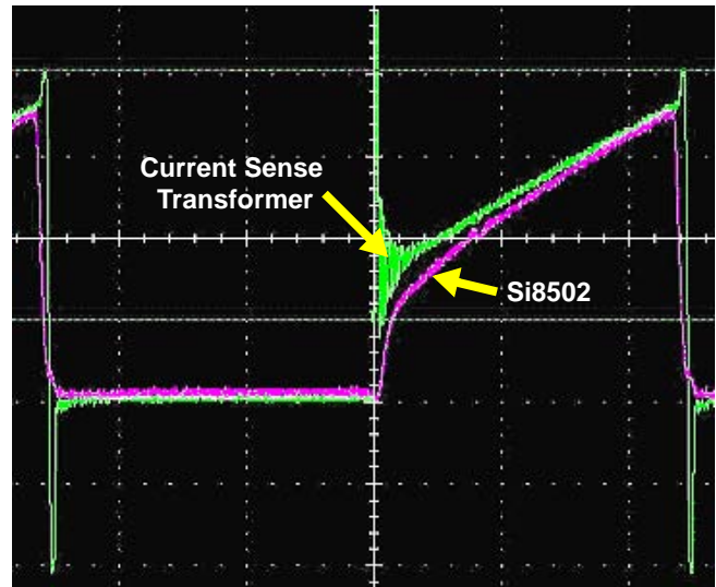
Figure 8. Leading-Edge Noise Suppression Waveforms (200 kHz, 9.3 A Load)
