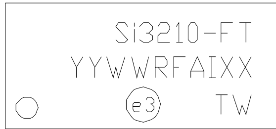
Figure 40. TSSOP Top Mark Diagram
