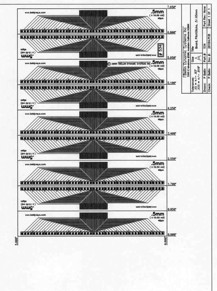
all 0.070" pads have 0.050" plated through holes on 0.100" grid ines between adapters grooved for easy snap-apart by hand
