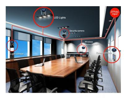
In order to reduce the use of energy a home or office building uses, smart solutions have been developed. These systems rely on programming and sensors in order to automate many processes in our homes and offices such as heating, cooling, and lighting.
