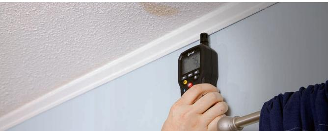
Everything you need in a meter for moisture remediation or HVAC: Bluetooth® METERLiNK capability, a pinless moisture sensor and pin probe, a temperature and relative humidity sensor, and an IR thermometer
