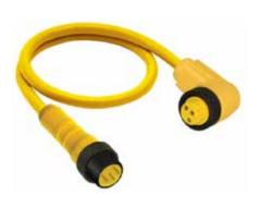
Mini, 7/8" double-ended cordsets, male straight with external threads to female 90° connector, 3-poles with molded cable, IEC color code.
