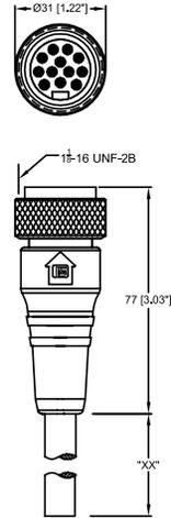
Mini, 1 1/8" single-ended cordsets, female straight, 12- and 19-poles with internal threads and molded PUR or TPE cable, Numeric color code.
