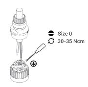
Unscrew the PE-contact, insert the PE-conductor and tighten again.
