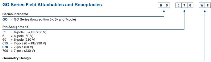
= 90° angled, female, (field attachable) = Male, PCB mount, (receptacle) FAV M = Male, octagonal flange, (receptacle) FA M = Male, rectangular flange, (receptacle)
