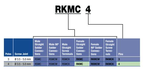
Table 15: Part Number Configurations for Pico M8 Field Attachable Connectors
