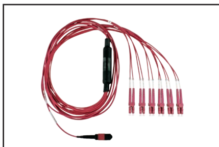
FP4LDMF003, FX Hydra Assembly, OM4, 6 LC Duplex, MPO-12 (female), Type-A Polarity 3 m
