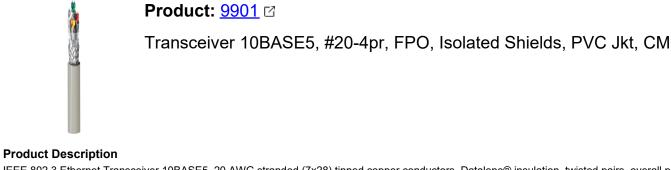
IEEE 802.3 Ethernet Transceiver 10BASE5, 20 AWG stranded (7x28) tinned copper conductors, Datalene® insulation, twisted pairs, overall polyester isolation tape + Duofoil® + tinned copper braid shield (95% coverage), drain wire, light gray PVC jacket.
