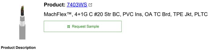
MachFlex™ for High Flex, 4+1G Conductor 20AWG (19x32) Bare Copper, PVC Insulation, Overall Tinned Copper Braid(85%) Shield, TPE Outer Jacket, PLTC
