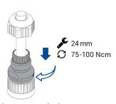
Screw the connector body to the contact holder.
