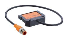
This AS-Interface Handheld controller serves to address the AS-Interface sensors, actuators and round cable modules. The mechanical connection is made by a mating M12 connector. AS-Interface flat cable modules are connected using the addressing adaptor type 0913 ATL 002/0.35 M. With this addressing equipment, all types of AS-Interface modules (including equipment with ASInterface Version 2.1) can be addressed.
