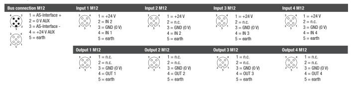
The connection to earth for the outputs is implemented via the earthing contacts at the fastening holes.
