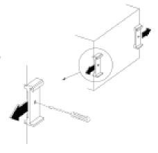
b. Push the SDN-PMBRK profile into the groove as far as possible. Secure with screw.
