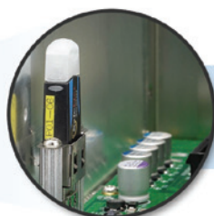
2. Withdraw the thumbscrew and remove the top cover
