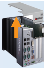
2. Withdraw the thumbscrew and remove the top cover
