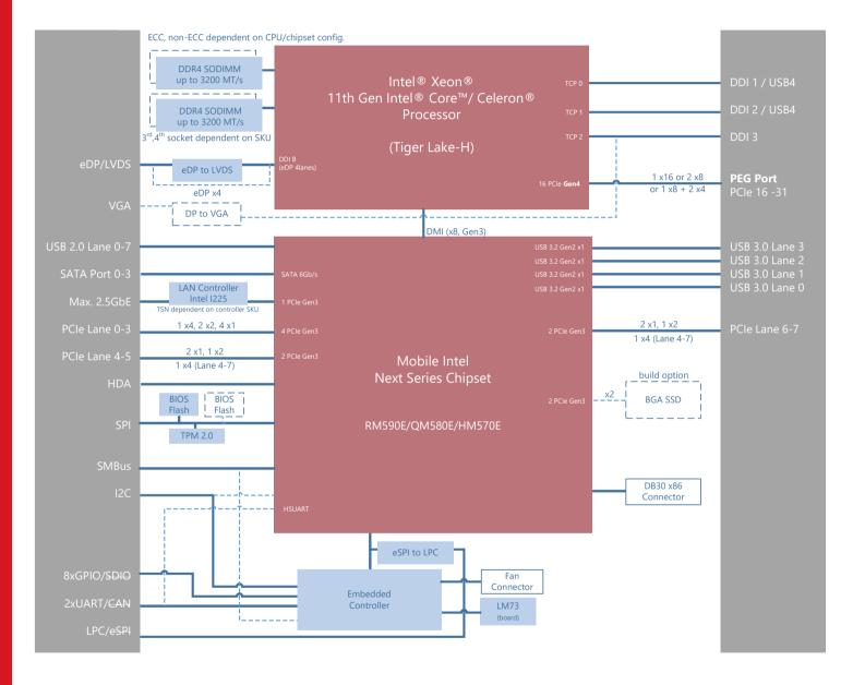
Note: "build option" indicates an alternative BOM configuration to support additional or alternative functions that are not available on the standard product. Be aware that these "build option" part numbers will need to be newly created and this will result in production lead times.
