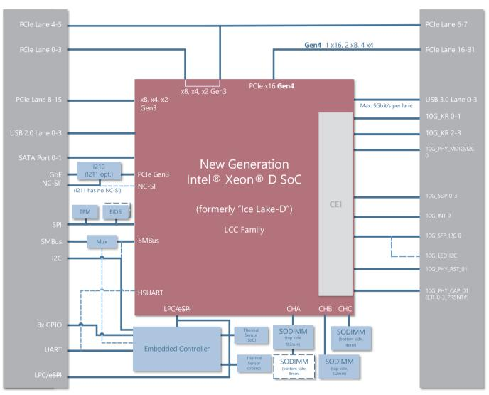
Additional PCIe x1 at Lane 1, Lane 5 is supported by project basis
