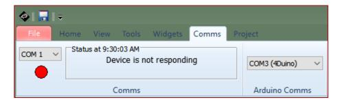
The Arduino Comms refers to the COM port that the Arduino board is currently using.
