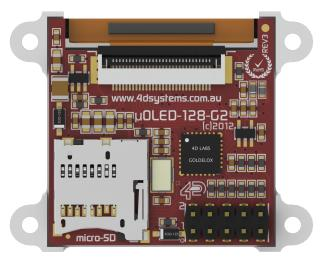
The **micro-SD** card slot on the module provides the user with expandable memory space suitable for multimedia file retrieval, including images, animations and movie clips, as well as data logging applications.
