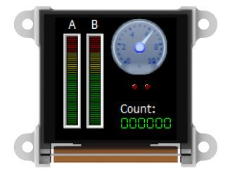
The **µOLED-128-G2** has a **1.5**" PMOLED Display at the forefront of the design that showcases the power and capabilities of the GOLDELOX processor. Combining a resolution of **128x128** pixels with **65K** True to Life colours, this display module is perfect for animations, slideshows and other multimedia presentations.
