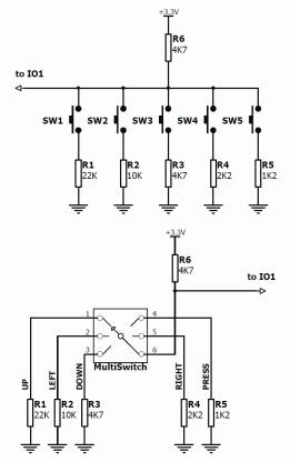
Unused buttons do not need resistors to be connected to the circuit. Table below lists the buttons and corresponding resistor values.
