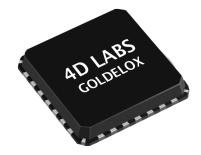
The GOLDELOX is a custom embedded graphics processor designed to interface with many popular OLED and LCD display panels. Powerful graphics, text, image, animation and countless more features are built right inside the chip. It offers a simple plug-n-play interface to many 8bit 80-Series colour LCD and OLED displays.
