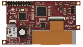
Audio support provided on the display module is supplied by the **PICASO** processor, an onboard audio amplifier and an  $8\Omega$  speaker. A simple instruction enables the user to play audio files while continuing the execution of the user application code, such as display updates, touch recognition, communications and much more.
