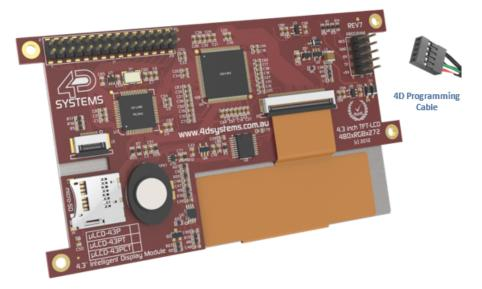
The PmmC file is programmed into the device with the aid of Workshop4, the 4D Systems IDE software (See Workshop4 IDE). To provide a link between the PC and the ICSP interface, a specific 4D Programming Cable is required and is available from 4D Systems.
