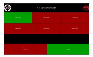
By default the resolution is 800x480. From testing at 4D Systems, resolutions up to about 1200x700 are perfectly usable, and anything beyond that requires knowledge of the system and a good eye, as fine text and icons can be difficult or impossible to read, especially when dealing with the higher resolutions.
