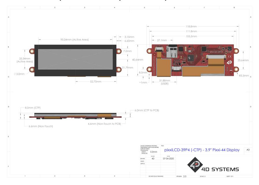
pixxiLCD-39P4 Series Schematic Details - REV 2.1
