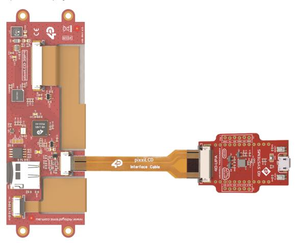
As shown, this connects to the pixxiLCD display through a 15-way-to-30-way cable.
