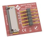
Alternatively, interfacing of the pixxiLCD display module can be done using a 15-way FPC directly to your product/project, without utilising the 15-to-30 FPC or the Interface board supplied. This would be the most efficient solution for a final designed product.
