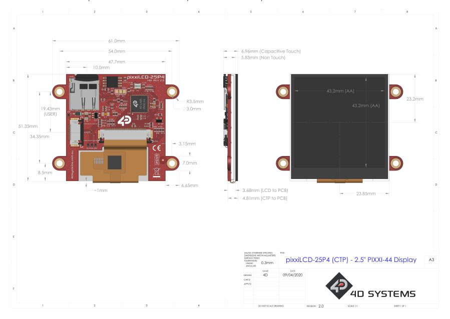
pixxiLCD-25P4 Series Schematic Details - REV 2.1
