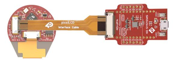
The 4D-UPA is used to update the PmmC and to download compiled 4DGL code into the processor. It also serves as an interface for communicating serial data to the PC.
