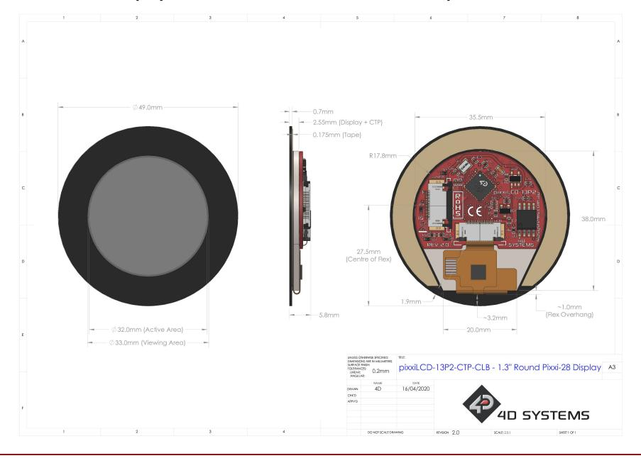
pixxiLCD-13P2 Series Schematic Details - REV 2.1
