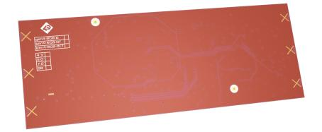
Where the Application PCB is shown to sit under the Application PCB Support section; can house a small metal shield of the same size. This shield is used instead of, or underneath an Application PCB, to aid the onboard electronics in the prevention of potential RF or EMI signals.
