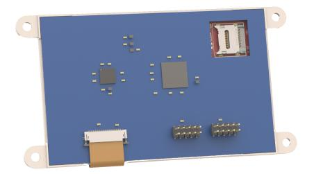
The 30-way FFC flex cable out of the gen4 into the application board can either turn up through a slot in the application board or can travel down under the gen4 plastic and emerge at the bottom and then into the application board (as depicted above).
