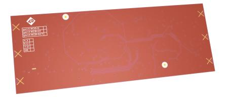
Where the Application PCB is shown to sit under the Application PCB Support section; can house a small metal shield of the same size. This shield is used instead of, or underneath an Application PCB, to aid the onboard electronics in the prevention of potential RF or EMI signals.
