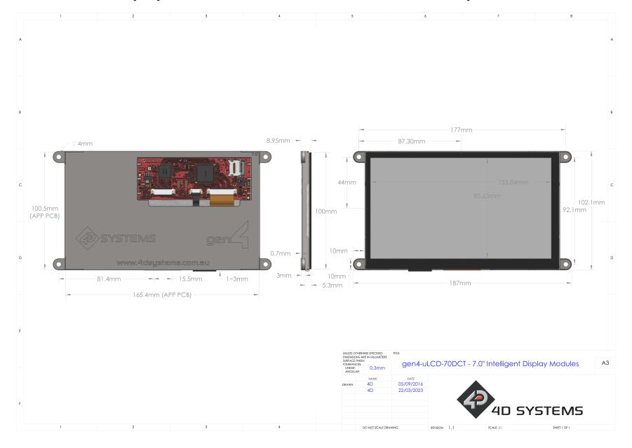
gen4-uLCD-70D Series Schematic Details (HW REV 1.2)
