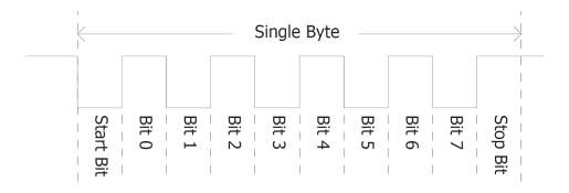
gen4-uLCD-70D Series Serial Ports - TTL Level
