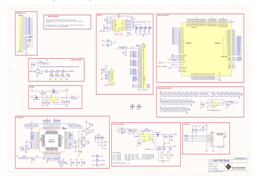
gen4-uLCD-70D Series Schematic Details (HW REV 1.3)
