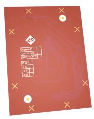
Where the Application PCB is shown to sit in under the Application PCB Support section; can house a small metal shield of the same size. This shield is used instead of, or underneath an Application PCB, to aid the onboard electronics in the prevention of potential RF or EMI signals.
