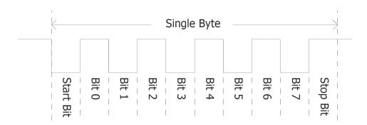
gen4-uLCD-32D Series Serial Ports - TTL Level Serial
