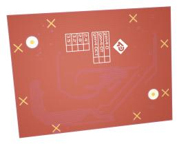
Where the Application PCB is shown to sit under the Application PCB Support section; can house a small metal shield of the same size. This shield is used instead of, or underneath an Application PCB, to aid the onboard electronics in the prevention of potential RF or EMI signals.
