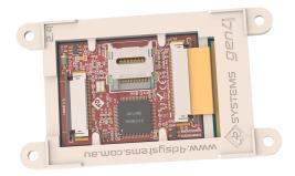
The image below (2.4" model depicted) shows a mock Application PCB on the back of the gen4 display (Blue area). It features a cut-out in the PCB so access to the micro-SD socket on the gen4's display board is possible, however, this may or may not be required depending on the application and if the micro-SD socket is utilised or requiring access once the Application PCB is applied.
