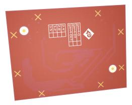
Where the Application PCB is shown to sit under the [Application PCB Support section; can house a small metal shield of the same size. This shield is used instead of, or underneath an Application PCB, to aid the onboard electronics in the prevention of potential RF or EMI signals.
