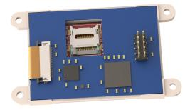
The micro-SD socket is a latch type, so it is accessible from the top, rather than a push/push or push/pull style which is accessible from the side.
