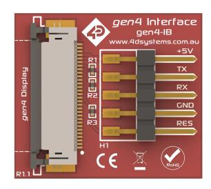
The gen4-IB can be used to interface with 4D Programming devices, as mentioned above, for interfacing to a breadboard for prototyping, interfacing to Arduino and Raspberry Pi interfaces (see gen4 -AR and -PI kits), or for interfacing to virtually any host.
