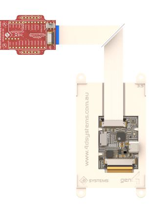
The 4D-UPA is connected to the ESP32 module using the supplied 30-way FFC Cable. The connectors on both the ESP32 module, and the 4D-UPA, are Top-Contact, meaning the FFC cable pins should be facing upwards, and the blue stiffener, should be facing down towards the PCB.
