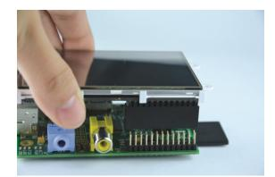
**NOTE:** The 4DPi-32 is supported only by the 26 way header, and therefore pressing on the touch screen may result in the 4DPi-32 moving towards the Raspberry Pi, and therefore the circuitry touching the Raspberry Pi. This could result in damage to either product if a short circuit were to occur. It is therefore highly encouraged to mount the display and attach the Pi to the mounted display.
