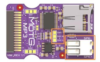
SPK+, SPK- provides a differential amplified output to a single speaker. Connect these pins to a 4/8/16/32 ohm speaker, at max of 3 watts when powered from a 5V supply. 8ohm 2.5W is recommended.
