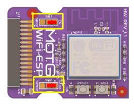
Unless the designer intends to use 2 UART MOTGs on a gen4-MOTG-AC2 board, the UART pins should be directed to TX, RX of the UMI as shown above.
