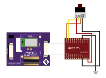
• While GPIO 9 of the gen4 PA is grounded, connect the GPIO10 (Reset) pin to Ground for a second and disconnect it (Reset) from Ground.
