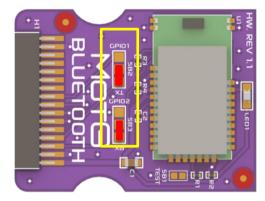
Unless the designer intends to use 2 UART MOTGs on a gen4-MOTG-AC2 board, the UART pins should be directed to TX, RX of the UMI as shown above.
