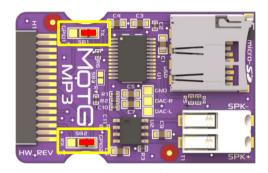
Unless the designer intends to use 2 UART MOTGs on a gen4-MOTG-AC2 board, the UART pins should be directed to TX, RX of the UMI as shown above.
