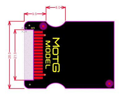
The MOTG boards are designed in such a way that the leading edge (header end) of the MOTG modules is a fixed design, and depending how complex the MOTG module is, will determine how long the board itself is. By default, the standard MOTG module is around 37mm in length, but can be extended longer if required. Note that depending on the target application, longer boards may have mounting challenges.
