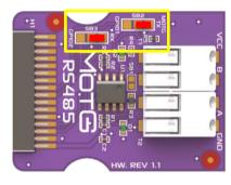
Unless the designer intends to use 2 UART MOTGs on a gen4-MOTG-AC2 board, the UART pins should be directed to TX, RX of the UMI as shown above.
