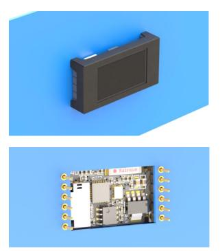
The IoD-09SM features surface mount castellated pads, and is designed to be soldered in place onto a host PCB. This module can be mounted on a PCB in 2 main ways.
