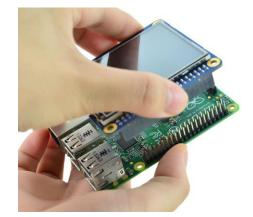
**NOTE:** The 4DPi-24-HAT is supported only by the 40way header, and therefore pressing on the touch screen may result in the 4DPi-24-HAT moving towards the Raspberry Pi, and therefore the circuitry touching the Raspberry Pi. This could result in damage to either product if a short circuit were to occur. It is therefore highly encouraged to mount the display on the Pi using standoffs (not supplied). Some options are available from places like Mouser.
