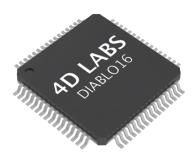
The DIABLO16 is a smart Controller and the interface to the TFT- LCDs is almost plug-n-play. All of the data and control signals are provided by the chip to interface directly with the display.
