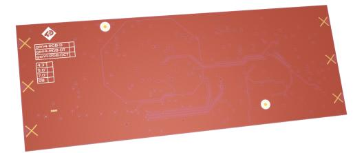
Where the Application PCB is shown to sit in under the Application PCB Support section; can house a small metal shield of the same size. This shield is used instead of, or underneath an Application PCB, to aid the onboard electronics in the prevention of potential RF or EMI signals.
