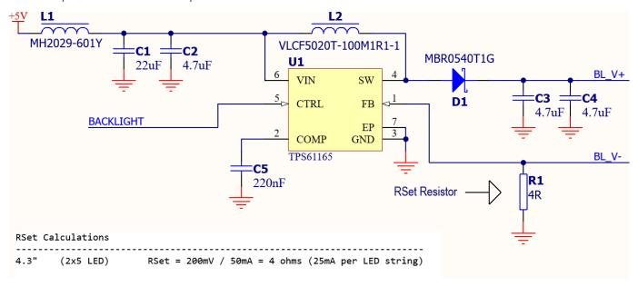
The RSet calculation is found in the Datasheet for the backlight driver. Each one will vary, as well as the circuit and the components required. Please refer to their datasheets.
