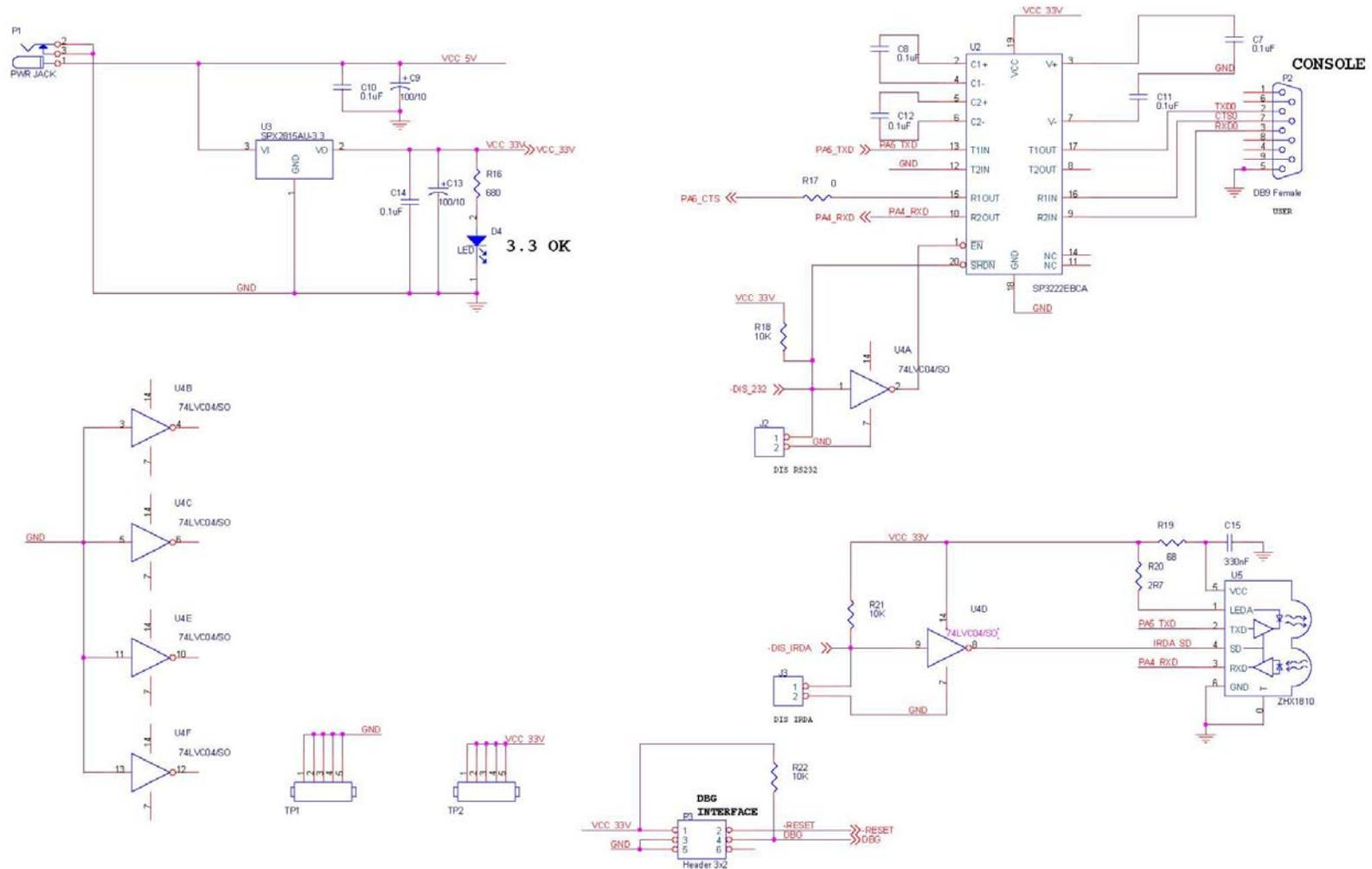
Figure 13. Z8FMC16 MDS Module (Power and Communications)
