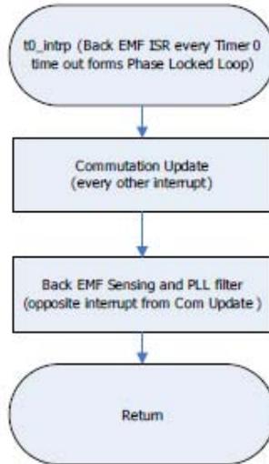
Figure 3. Back EMF Sensing Phase Locked Loop
