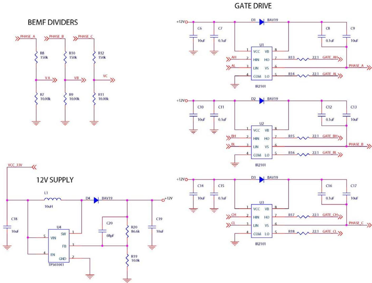
Figure 10. 3-Phase MotorControl Application Board (Part 2 of 3)
