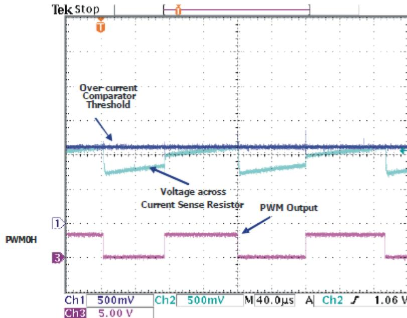
Figure 8. Cycle-by-Cycle Shutdown
