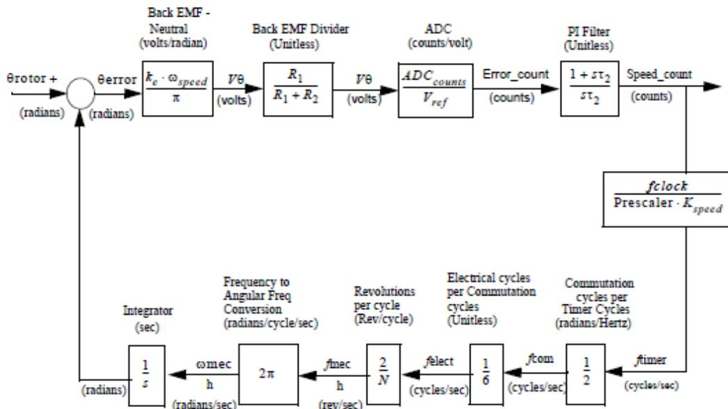
Figure 4. Back EMF Sensing Phase Locked Loop
