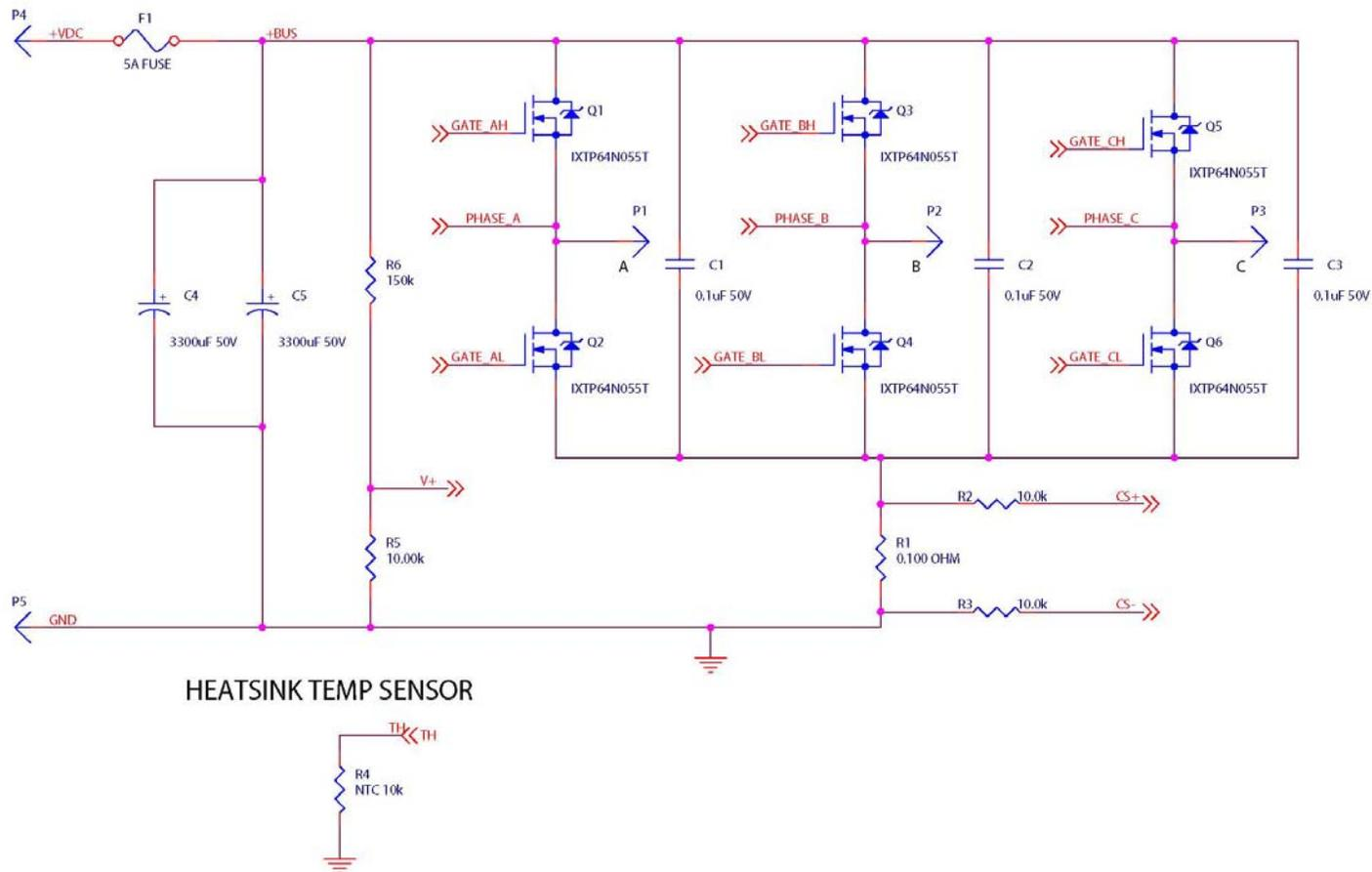
Figure 9. 3-Phase Motor Control Application Board (Part 1 of 3)
